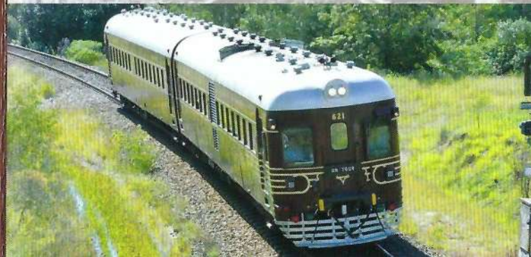
(Below) The last surviving 600-class units. The 600 Class 2-car units were introduced in 1949 for country service. Constructed principally of aluminium, they represented a new era of rail motor design in NSW.
