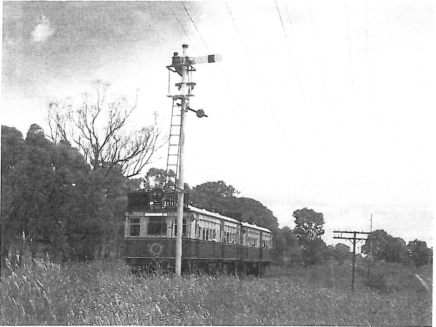
WR71 stands at the Down Home signal at Kandos while safeworking duties are carried out as the points are set for the cement siding. This signal is rarely cleared for passage towards Mudgee and this is one of those occasions. Rail services have been temporarily suspended from Kandos to Gulgong since 2007.
