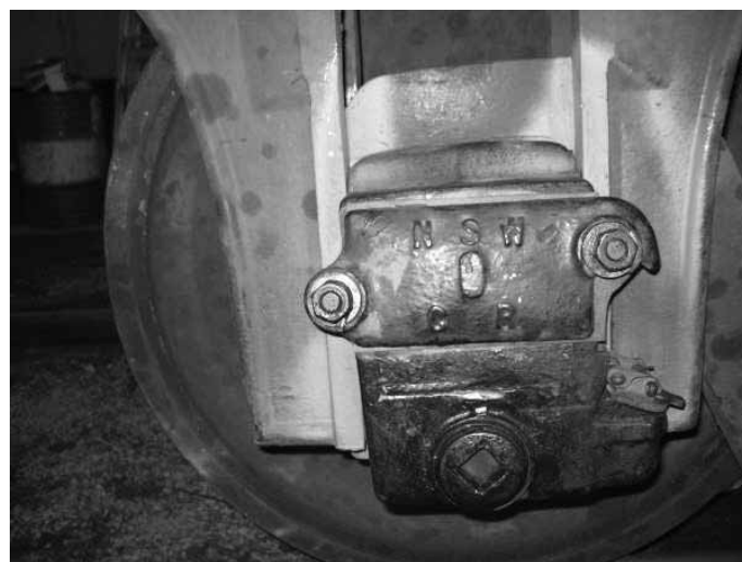
Reconditioned axle box fitted to journal.
