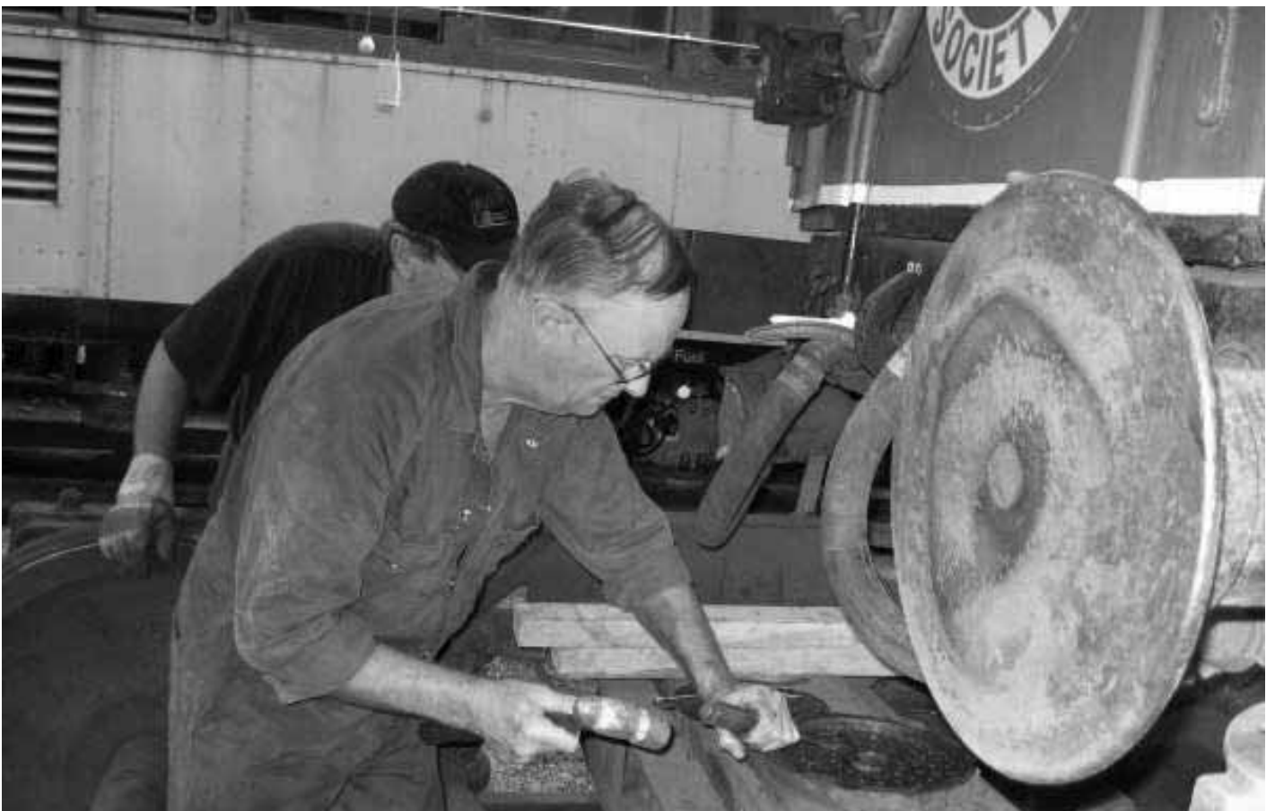
Stafford makes final adjustments to the wear plate in the queen casting.
