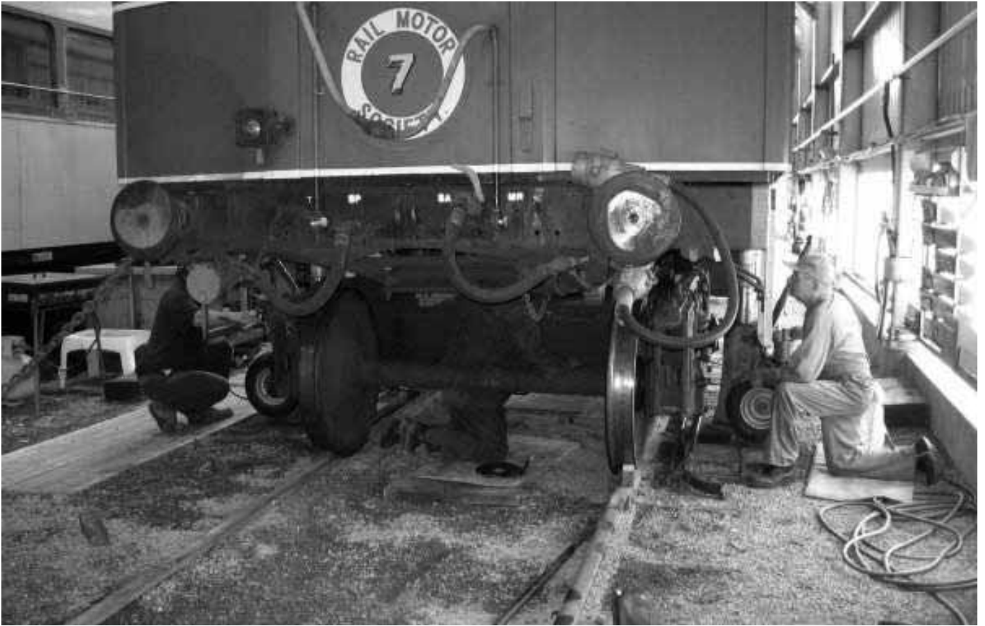
CPH 7 is supported on hydraulic jacks ready to lowered onto the overhauled bogie.
