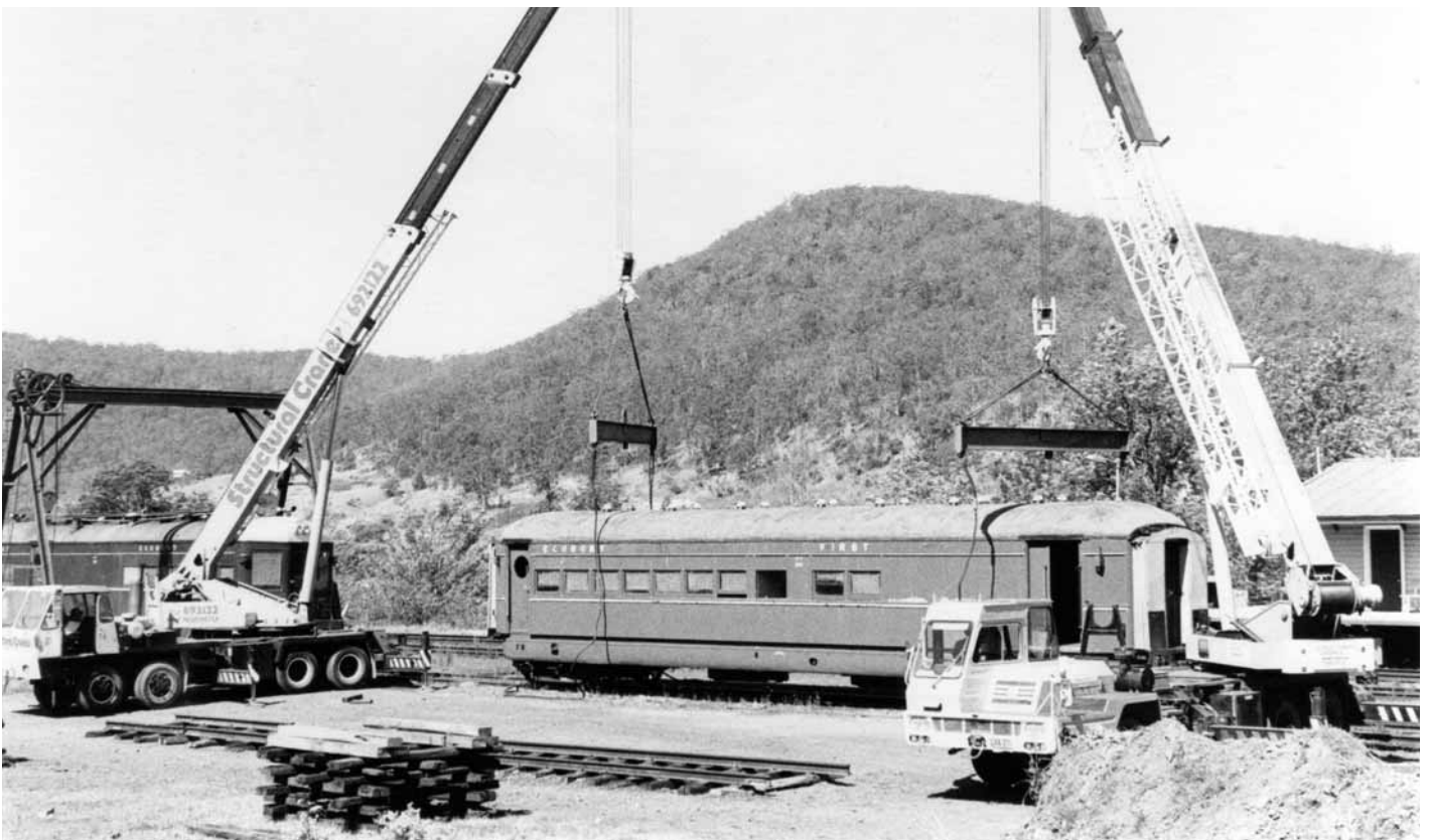
HPC 402 and HCT 502 were dead-hauled from Werris Creek on 7th October, 1984. HCT 502 was purchased for parts to complete FT 501, which was purchased from Carriage Works (Eveleigh) in refurbished condition but lacking bogies and skirts. The body of 502 was lifted without bogies onto styes (pictured in foreground) for stripping, after this was completed the remaining body was hauled by road to the Dorrigo Steam Railway Museum. Photo: Geoff Murray
