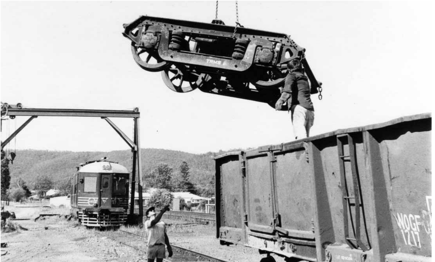
The bogies used to transport CPH 14 and HCT 502 were returned to Sydney in a bogie open wagon supplied for the purpose. Members Mick Turton and Bruce Harris are loading the last bogie from 502 which eventually returned to Paterson under FT 501. HPC 402 can be seen waiting its turn with the mobile cranes under the former goods yard crane.
