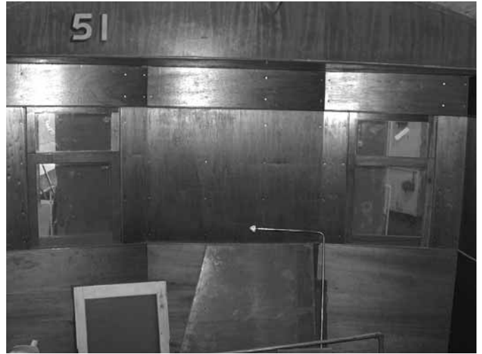
Non-driving(No.1) end re-lined and fitted with new windows.
