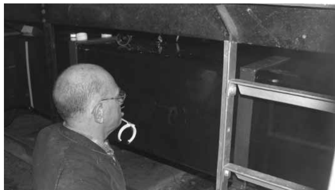
Bryan Hicks fitting the retention toilet tank to CPH 3.
