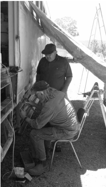
(Clockwise from top left) Trailer 729 has had its whiskers masked and awaits the application of a glossy coat of Indian Red paint to finish the job; Project Sputnik painter Pete progresses with the tedious job of masking the end lining on 729; 621/721 preparation for painting; body repairs underway.
