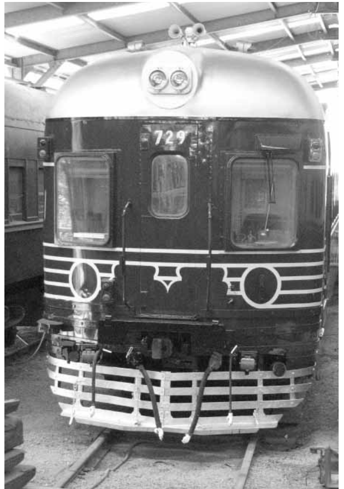
(Clockwise from top left) Trailer 729 has had its whiskers masked and awaits the application of a glossy coat of Indian Red paint to finish the job; Project Sputnik painter Pete progresses with the tedious job of masking the end lining on 729; 621/721 preparation for painting; body repairs underway.
