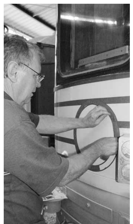
(Clockwise from top left) Trailer 729 has had its whiskers masked and awaits the application of a glossy coat of Indian Red paint to finish the job; Project Sputnik painter Pete progresses with the tedious job of masking the end lining on 729; 621/721 preparation for painting; body repairs underway.
