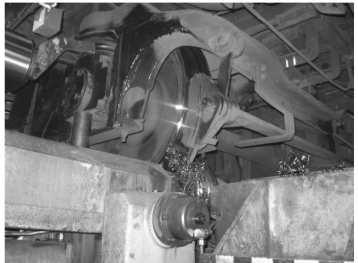
Cutting of another wheel is underway and the metal “swarf” shavings which are the removed wheel metal can be seen curling near the cutting tool.
