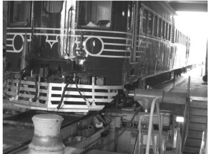
Positioned on the wheel lathe at DELEC, the lathe operators commence machining of the first of 621's wheels. Using ropes, the capstan wheel in the left foreground can be used to reposition vehicles on the lathe.
