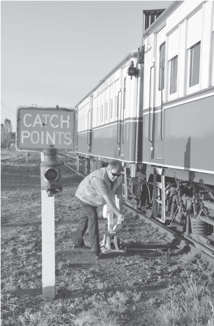
Ensuring the safe exit from Junee depot, Doug Bennett has a firm hold as the CPHs pass over the catchpoints which prevent runaways from the depot to the main Junee yard. Photo: S. Preston
