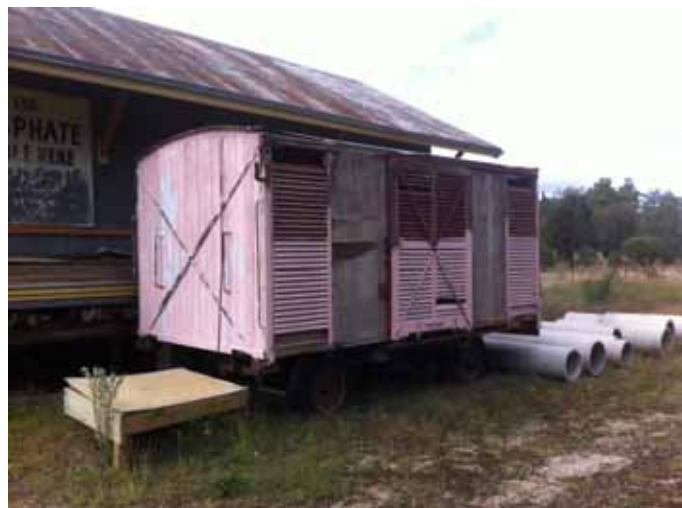
Ladysmith 2012: The restoration of GT 73's body is well underway by Tumba Rail at Ladysmith, NSW. Plans are already in place to replace its current rubber tyred "Blitz Truck" underframe with a more appropriate rail type. Photo: Bob Gioia
