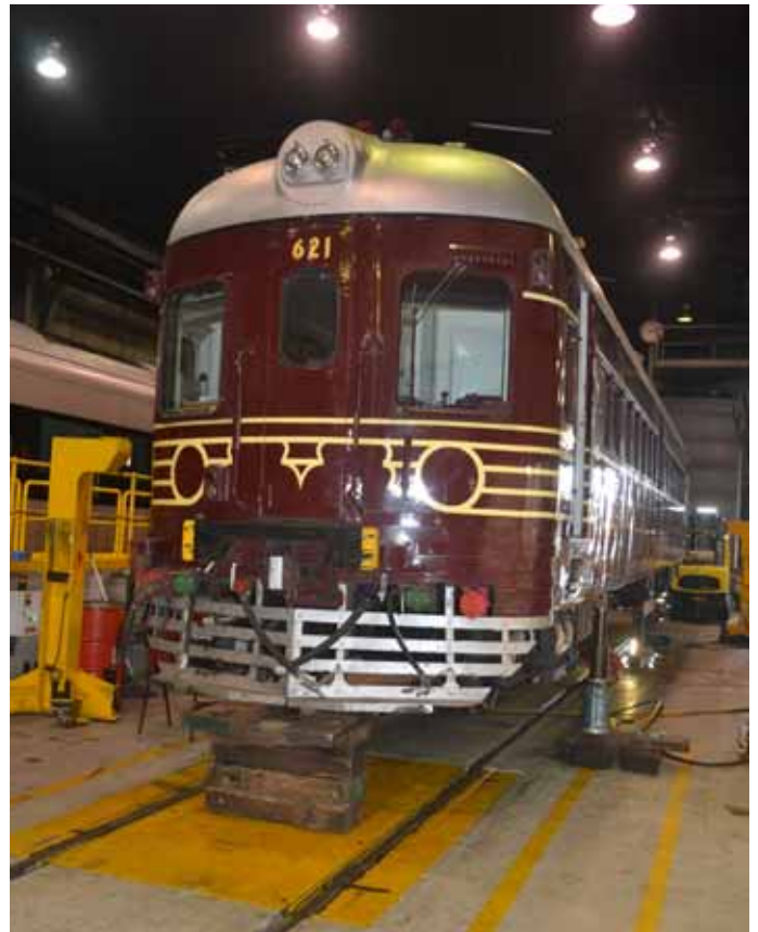
621 is supported on jacks for the change-out.
