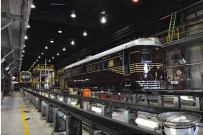
With the lift and engine swap completed 621 was placed on the No.3 high stand road to facilitate the reconnection of engine attachments. In the photos above (left) 621 stands separated from its trailer in the company of Hunter car 2705 Greg Gooley (right) is seen offering up the exhaust to the refitted motor.
