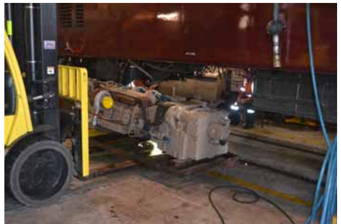
The replacement engine and transmission are lifted into place by a forklift.
