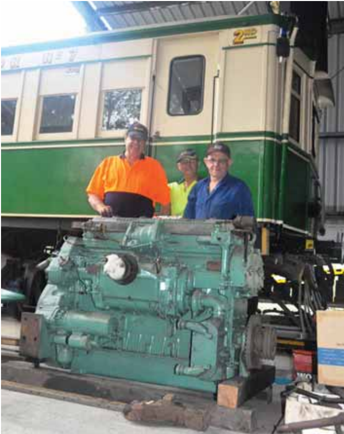
Standing behind the reconditioned GM 6-71 diesel engine destined for HPC 402 are (L to R) Bruce Agland, Stafford Payne and Bryan Hicks. Photo: SG Preston
