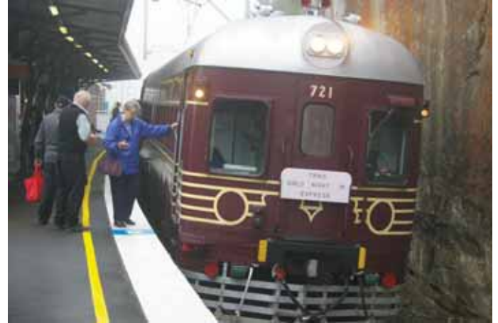
721 has stopped at Leura platform to collect its returning passengers, the rust stained cutting above showing the effect of the heavy braking by freight trains which is required to retard their run down the grade.
