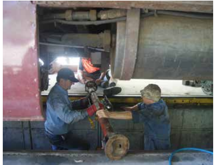
With the lift finished the reconnections commence including the drive shaft which Mick and Bryan prepare to man handle into place between the transmission and final drive. Photo: Steve Davies
