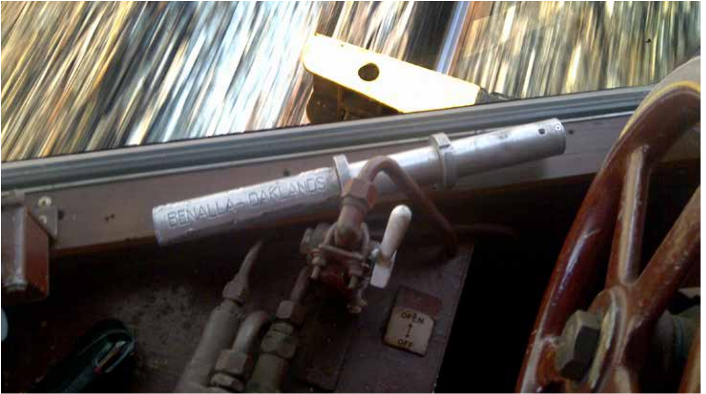
The Ordinary Train Staff clearly shows the section names authorised for travel and having being handed to the driver, 402's trip along the Oaklands line has commenced. Photo: S. G. Preston
