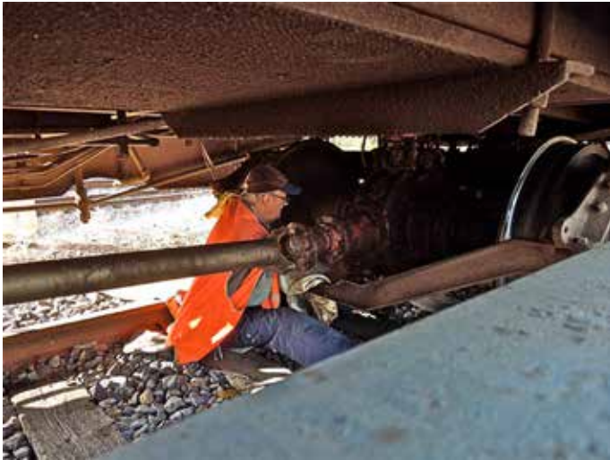
Throughout the journey the Society's Engineering Manager and travelling fitter for the trip, Stafford Payne, monitored all aspects of 402's performance including a troublesome final drive seal. An early evening arrival at Seymour loco depot provided a suitable and safe opportunity for Stafford to get his hands dirty and inspect the seal to ensure that its condition had not deteriorated. Photo: Spencer Ross
