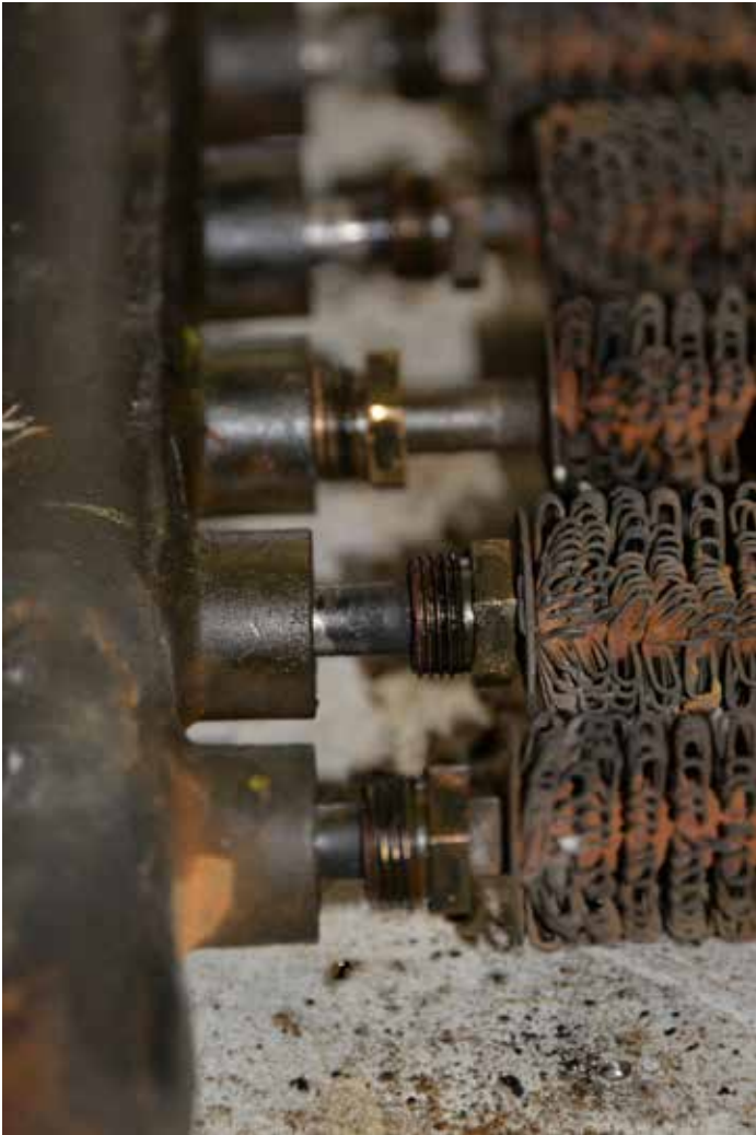
The overhaul of 402's radiators requires 800 of these radiator connections to be undone and the seals replaced before reinstallation. (Photo: SG Preston)
