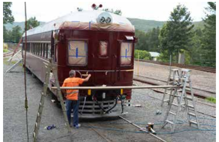
After a brief drying period Pete peels off the masking to reveal 721's untouched cream whisker lining hidden beneath the tape and top coat. (Photo: Bruce Gehrig)
