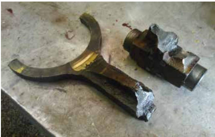
The broken nature of CPH 3's crown wheel fork is clearly evident in this picture taken upon return to Paterson. (Photo: Bruce Agland)
