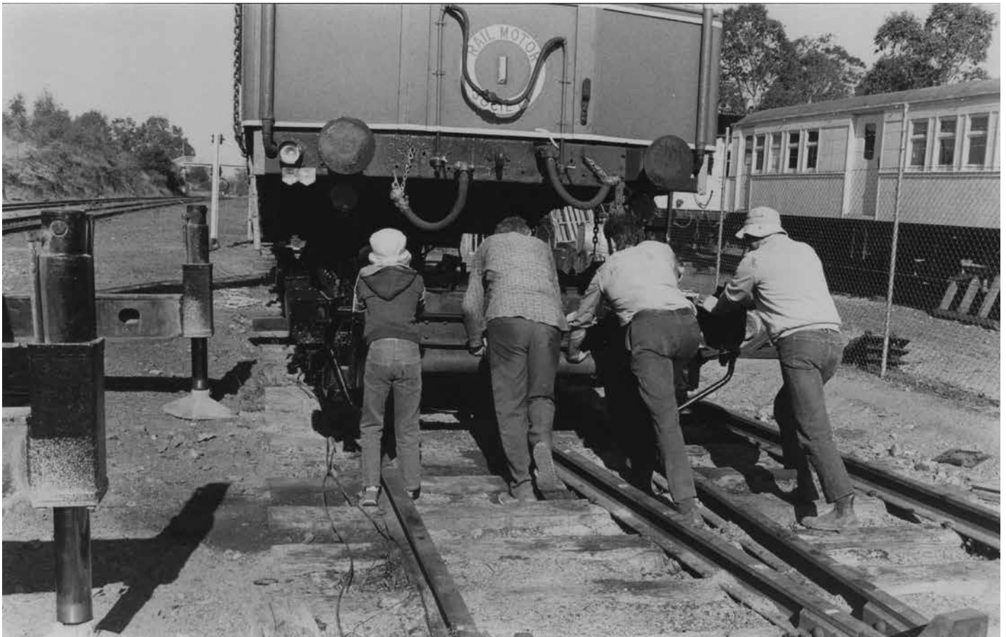
(Above) Pigstyed on timbers CPH 1 awaits the arrival of the road crane. (Below) The combined strength of Glenn Davies, Graeme Bedwin, Bruce Kingsford and Steve Davies carefully place the No1 end bogie back under CPH 1 which is suspended by the road crane. (Photos: Geoff Murray)
