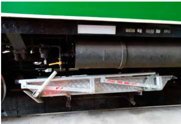
The new steps in their storage position under CPH7. (Photo: M. Walsh)
