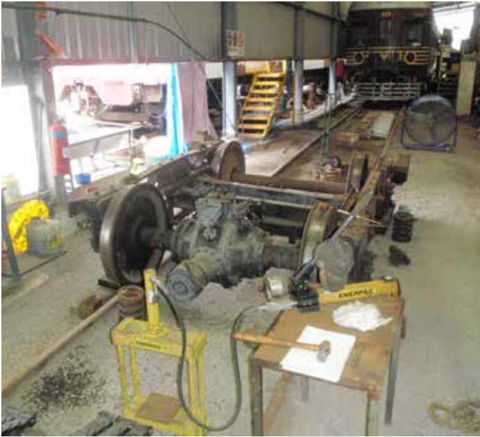
CPH 3 has been lifted within the Paterson shed to allow inspection and testing of the primary and secondary springs. (Photos: Bruce Kingsford)
