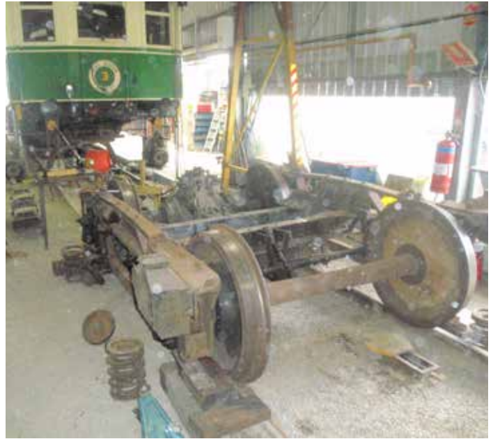
CPH 3 has been lifted within the Paterson shed to allow inspection and testing of the primary and secondary springs. (Photos: Bruce Kingsford)
