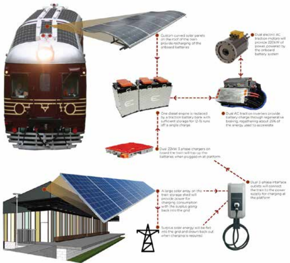
A diagram of the main components of the solar train concept. (Image: Byron Bay Railroad Company)
