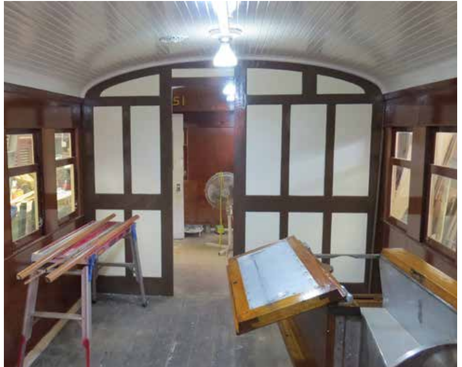
CTC 51 is starting to return to its former glory with the interior being painted and the original water cooler being restored in the foreground. (Photo: Jan Oxford)
