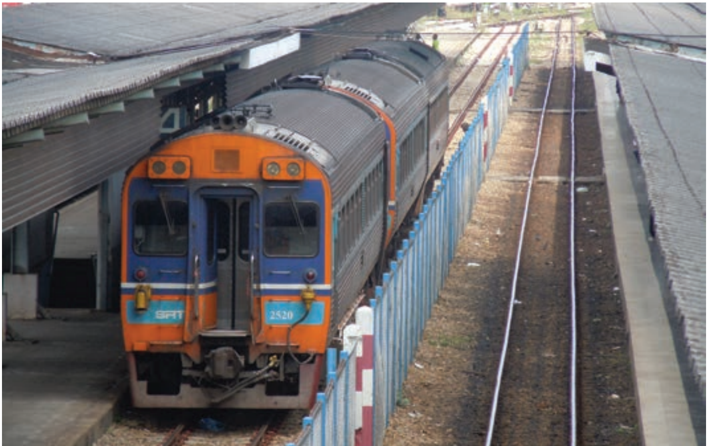
Long-time member, Warren Mills, captured this 3 car railmotor set at Hat Yai in southern Thailand, close to the Malaysian border. The State Railway of Thailand (SRT) operates a metre gauge network of over 4000 km and uses many railmotors, such as this air-conditioned APD 20 set built in South Korea in 1995 by Daewoo Heavy Industries. (Photo: Warren Mills)
