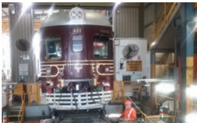
John operates the pneumatic "Mule" to move 621 onto the Wheel Mill at Flemington. (Photo Mick Walsh)
