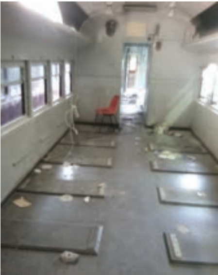
Seats removed showing the interim seat bases placed some years ago to support the seats. (photo TRMS)
