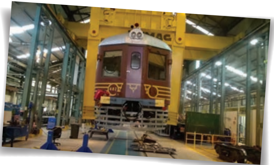
Above and below 402 being lifted clear of its Bogies. (photos UGL).
