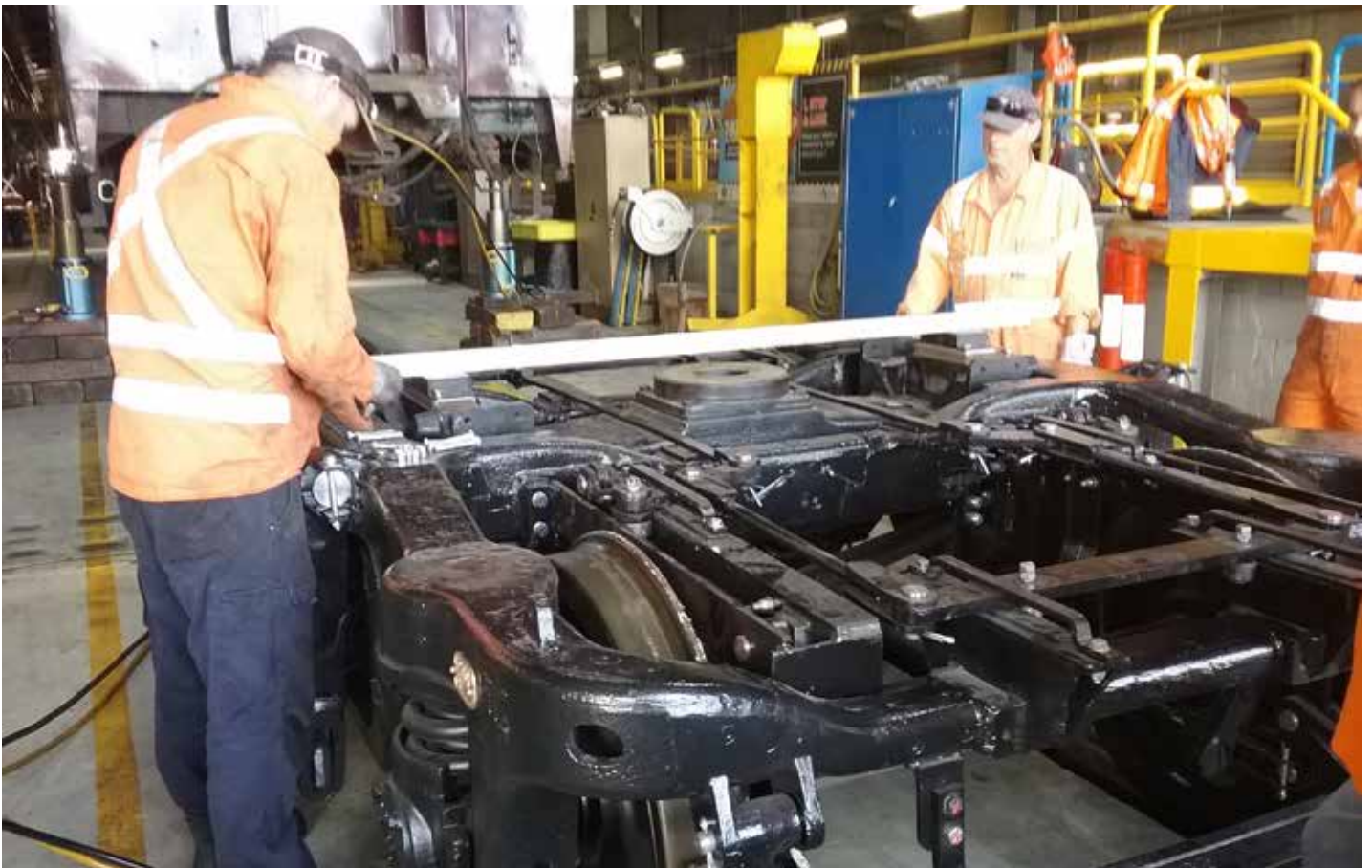
A new bogie is readied prior to fitment to 721 at Broadmeadow Service Centre. (Photo: Mick Walsh)
