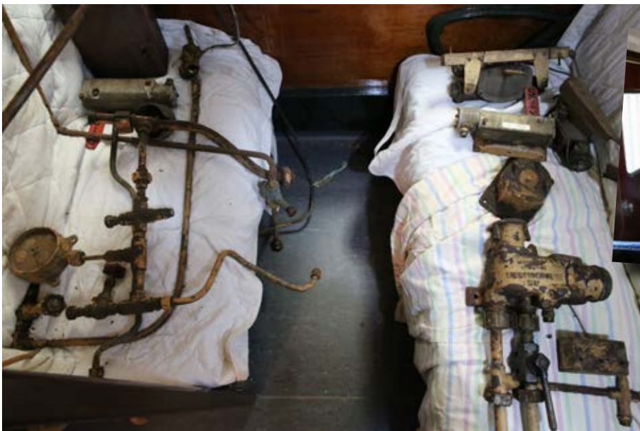
Parts salvaged from CPH 14 are ready to be installed in CTC 51 driver's cab
