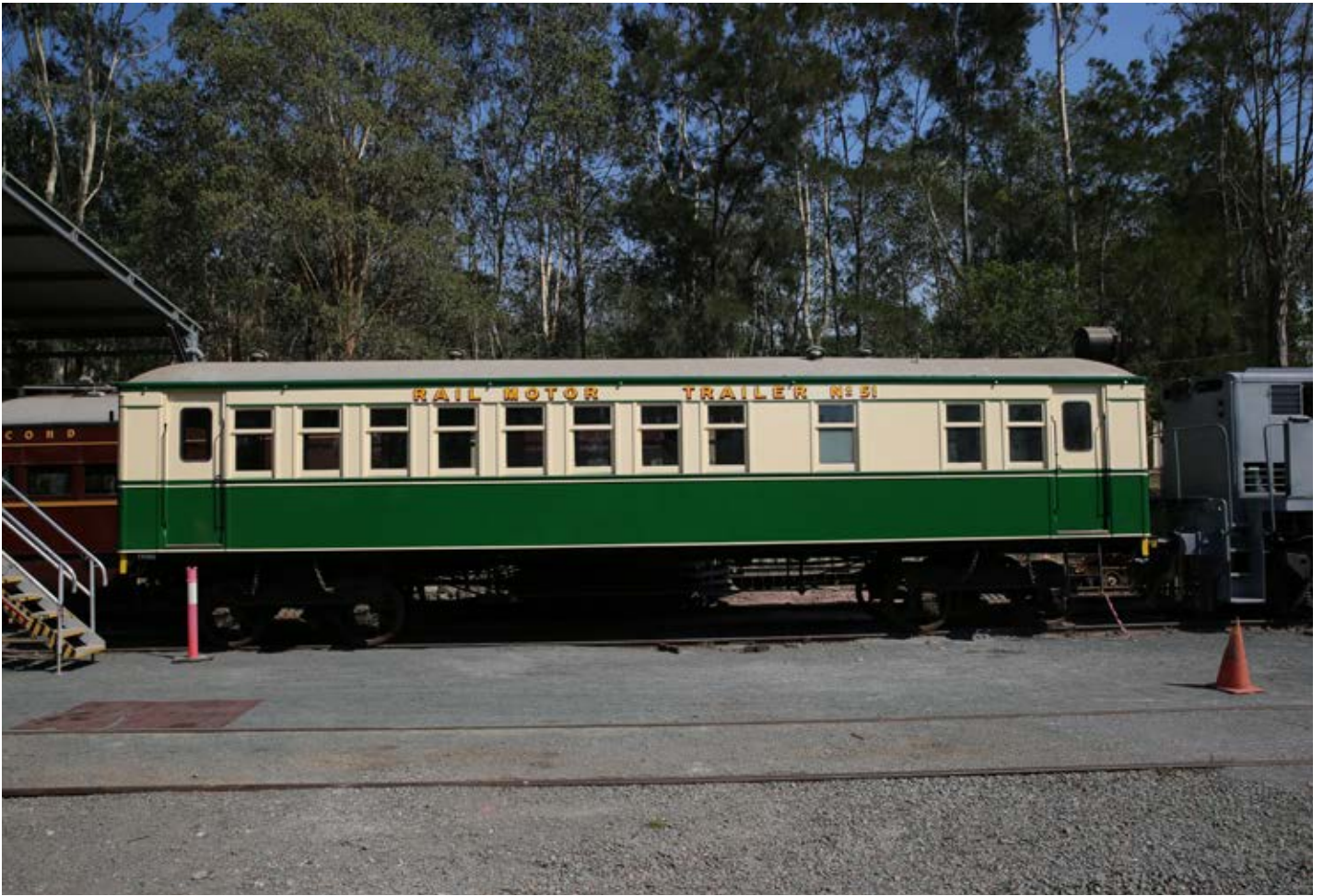
Top: With a fresh coat of paint and letter boards affixed, CTC 51 outwardly looks set for action. However the reality is that although most of the work 'above floor' nears completion this only signals the start of considerable work 'below floor' on wheels, bogies, brake gear, etc.
