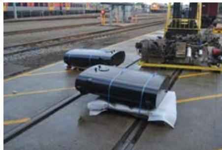
New fuel tanks with old engine in the background. Photo Bruce Agland
