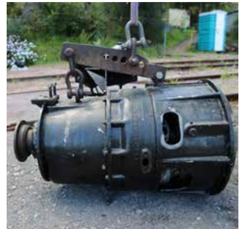
The recently failed Twin Disc transmission after removal from CPH 1
