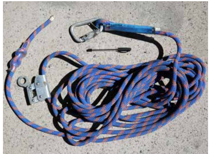
Portable overhead safety line
