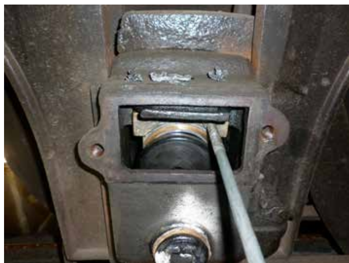
CPH 1's axle-box is inspected for wear and serviced by Steve Watt. The axle-brass can be seen in the centre.
