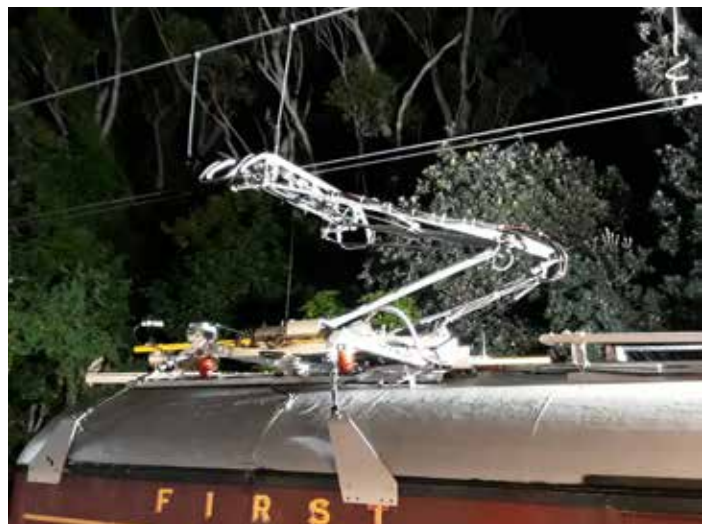
Pantograph in operation at night (Bruce Agland)
