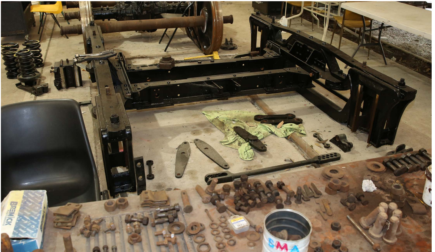
A pair of 2QG bogies await reassembly
