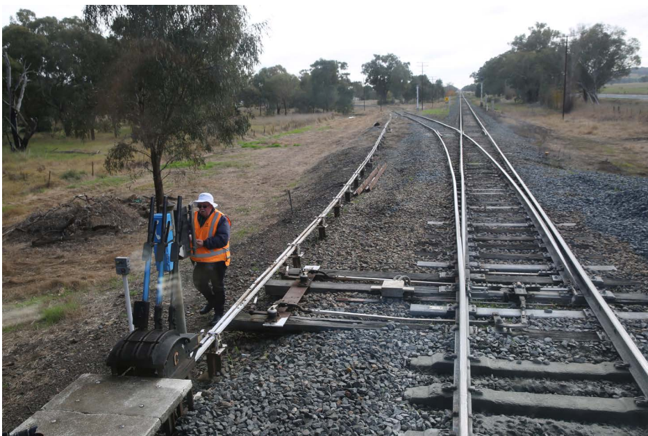
621/721 has just come off the Rand line (left) where TRMS driver Phil Smith resets the points to the main line running (R Spencer)
