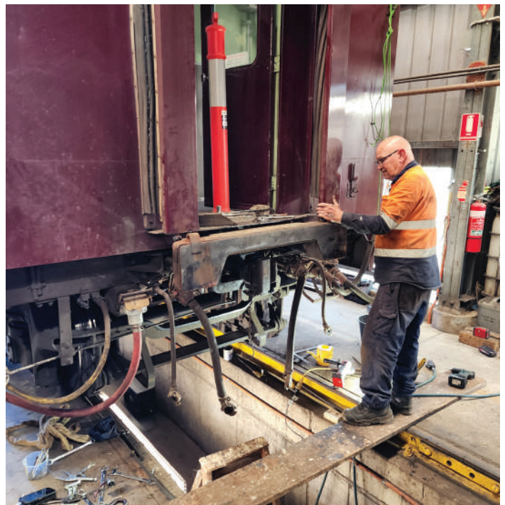
Kevin Judd and Ross Goodman (out of shot) reinstall 721's rear auto-coupler, plunger bar and buffer beam after making repairs to mitigate unwanted noise, 5 Dec 2023 (Robert Spencer)
