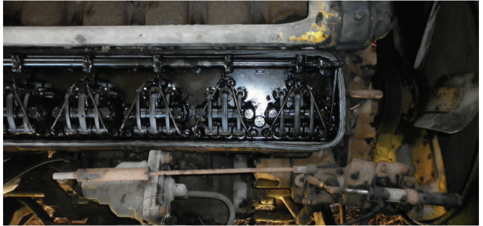
Looking down on the Detroit engine in 602, with its rocker cover removed, 15 Feb 2023. Grahame Pantin is about to remove the diesel injectors for cleaning, before an attempt can be made to restart this engine
