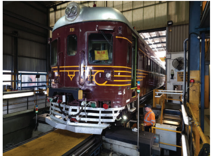
721 is positioned onto the wheel mill using a “mule” controlled by Mill Operator, John Wilson
