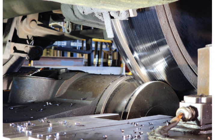
The wheel rotates slowly in a grooved roller while the milling head cuts into the wheel at high speed from below. Metal shavings are visible.
