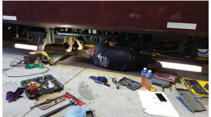
The diesel injectors in 621's No.1 engine receive much needed attention in the expert hands of Adrian Tanner, during an engine "tune-up", 6 Dec 2023
