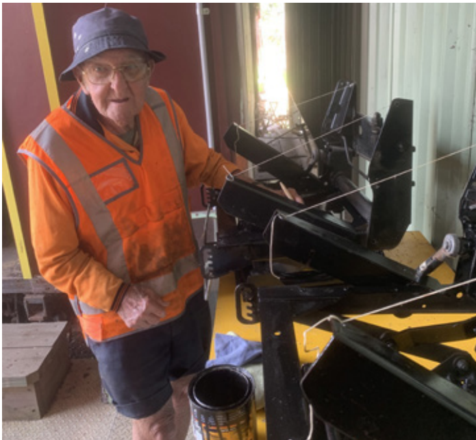
Ted Dunbar applies black paint to two driver's seat frames. The refurbished seats will be installed in 629/729.
