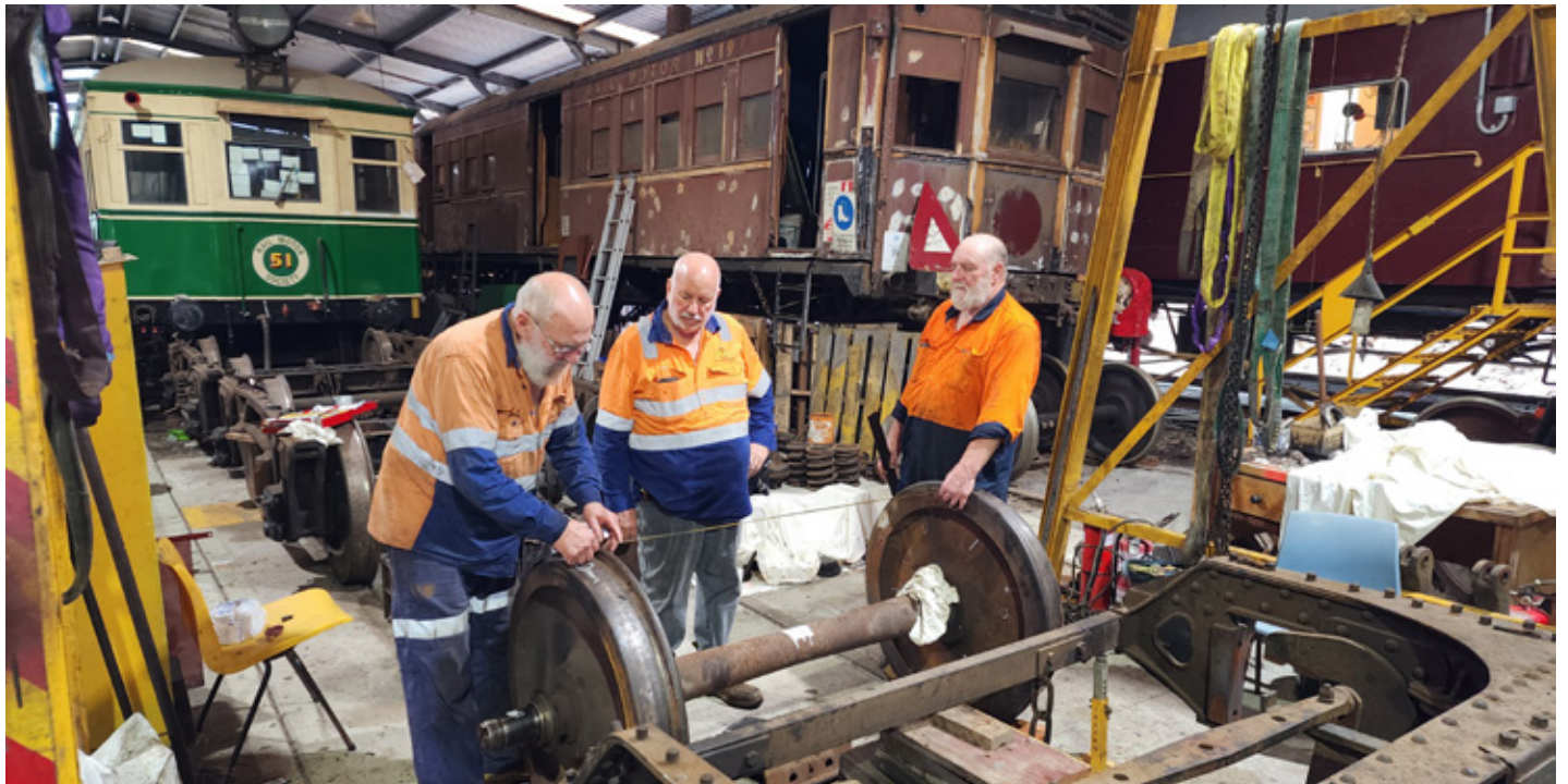
Above: Ross Goodman and Mark Bennett carefully measure the inside wheel distance at four quadrants on 402's leading wheelset, checking for any variations, as Rod Short watches on.
