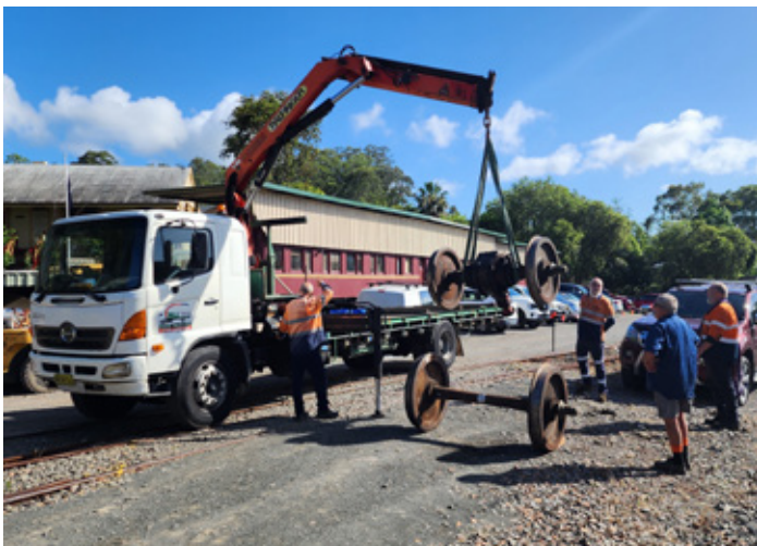
402's wheelsets are shown being loaded for transport to Sulzer's Service Centre at Maitland, where they will be machined to restore the tyre profile.
