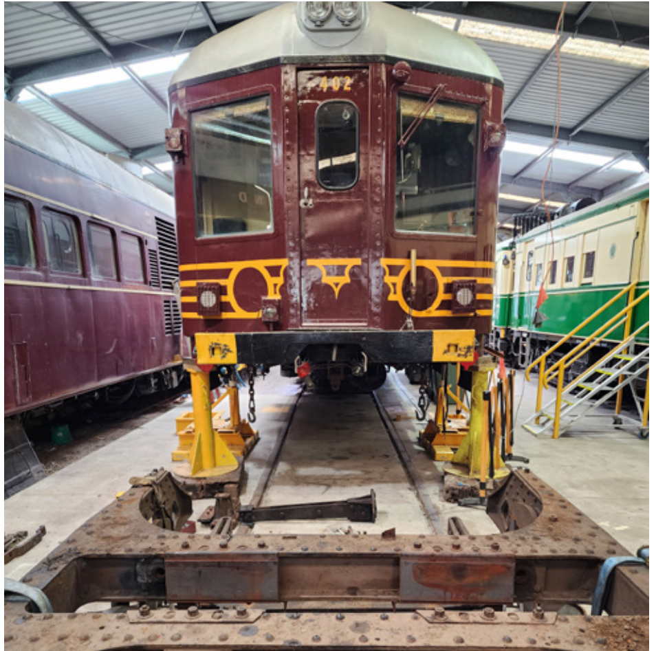
HPC 402 is supported on stands to allow its leading bogie to be removed and stripped down for remediation.
