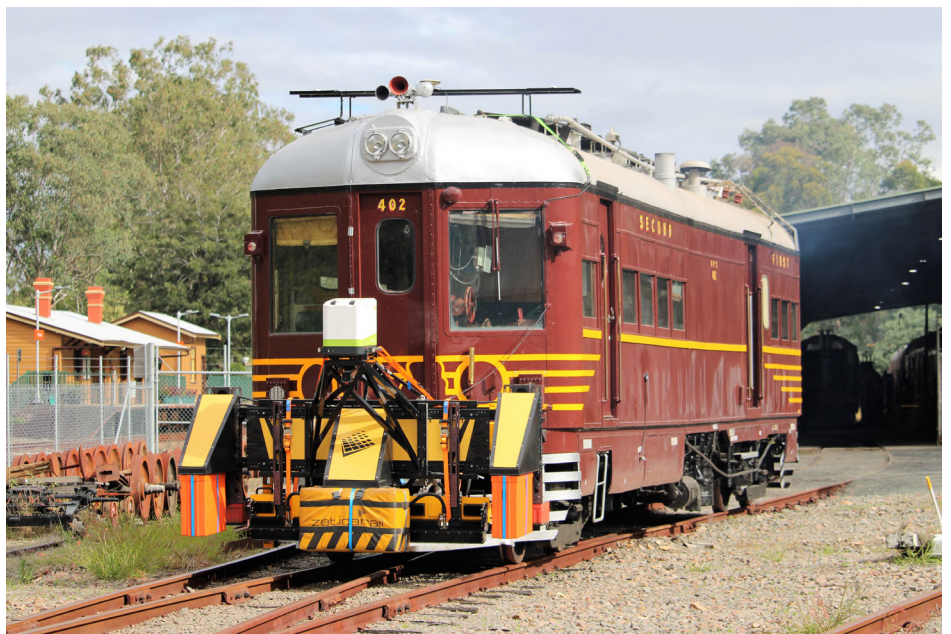
HPC 402 with GPR equipment installed (B. Gebrig)
