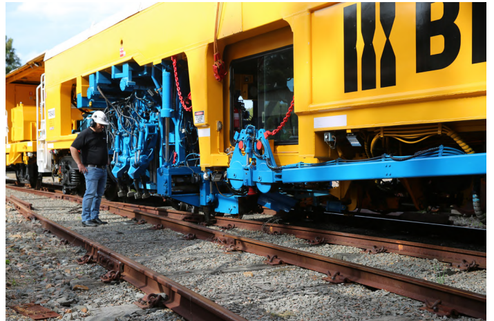
On Sunday 16 April, after its successful Community Event concludes, Brimble's TMS400 Turnout Tamper machine straightens track within the depot precinct before leaving, courtesy of Brimble Rail (R. Spencer)
