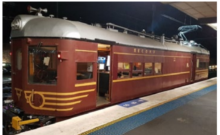
402 at Waterfall, with pantograph raised, performing overhead wire testing in 2022 (Bruce Agland)
