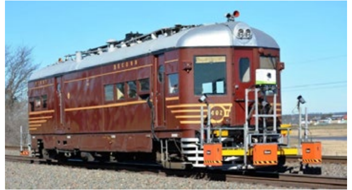
402, now owned, restored and operated by the Society, as seen in 2016 near Farley with ground penetrating radar attached for ballast testing. It also performs radio testing for ARTC and overhead wiring checks for Sydney Trains in new and unusual roles (Bruce Gehrig)
