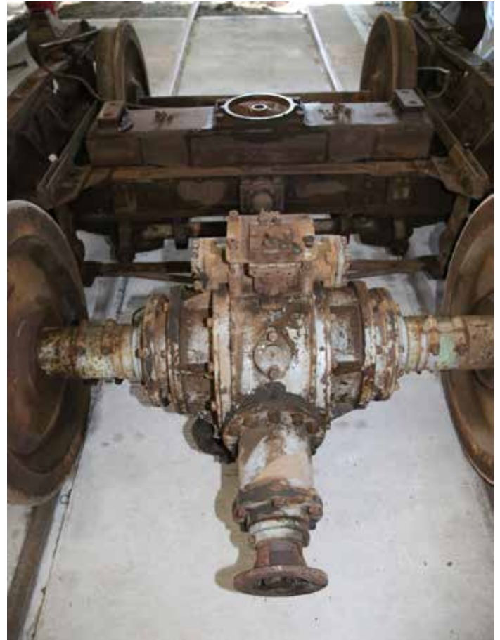
Drive bogie recovered from CPH 19 ready to be stripped for overhaul.
