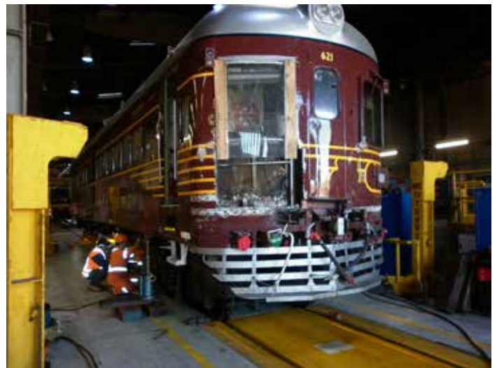
621 being lifted at Broadmeadow Maintenance Centre to check front bogie for damage.
