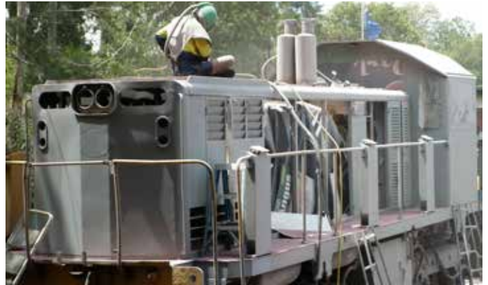
Sandblasting in progress.
