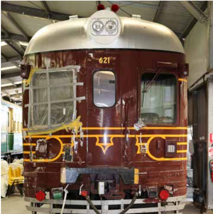
621 on return to Paterson. Note the displaced front buffer beam, patched guard's window and damaged or destroyed train fittings.
