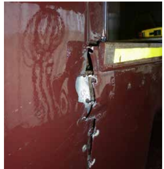
Rivets have been ripped out and the aluminum skin has buckled outward below driver's side door. The vestibule floor and brass edging strip were displaced outward.
