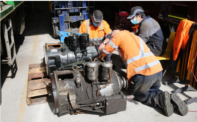
Out with the old and in with the new, as Mick, Kevin and Mehdi prepare to install our recently overhauled spare transmission in CPH 3
