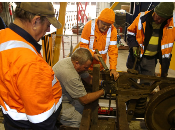
Volunteers dismantle one of the bogie frames removed from CPH 19 under the watchful eye of Bruce Agland
