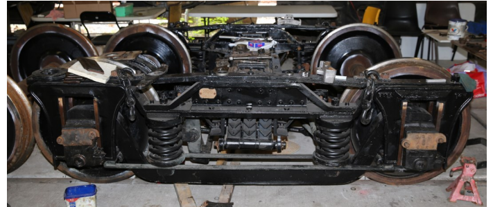
CPH bogie in late stages of reassembly following heavy overhaul (Dec 2022)
