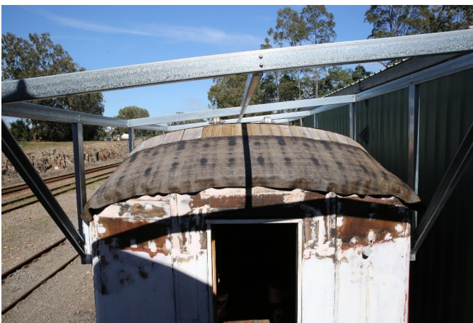
Malthoid fitted to the roof end of the goods van. Photo: Robert Spencer
