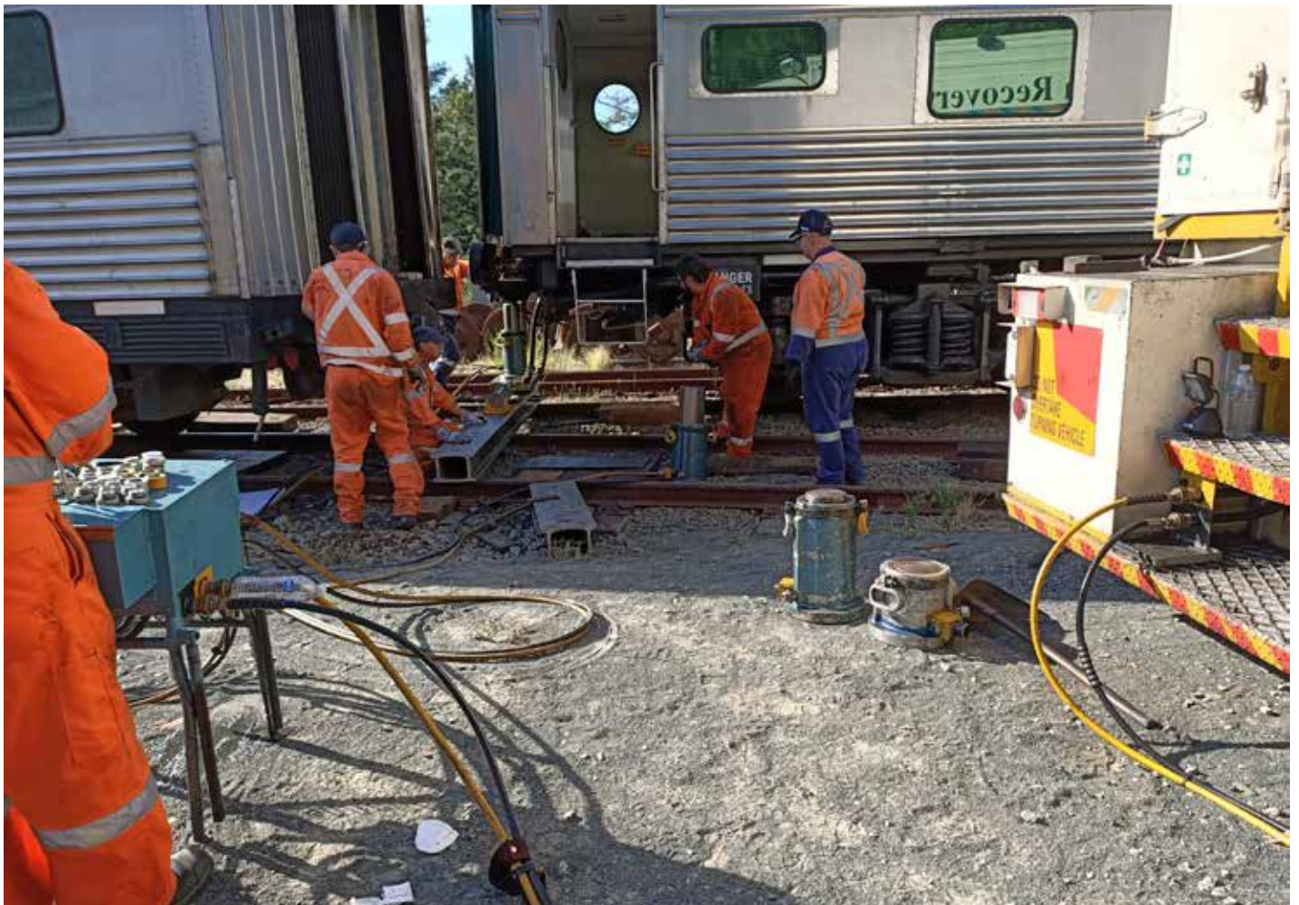
Unusual visitors to our Depot Yard, Sydney Trains' Emergency Train Recovery Unit personnel rerail Southern Aurora cars on 16 Mar 2022 (Warwick Erwin)
