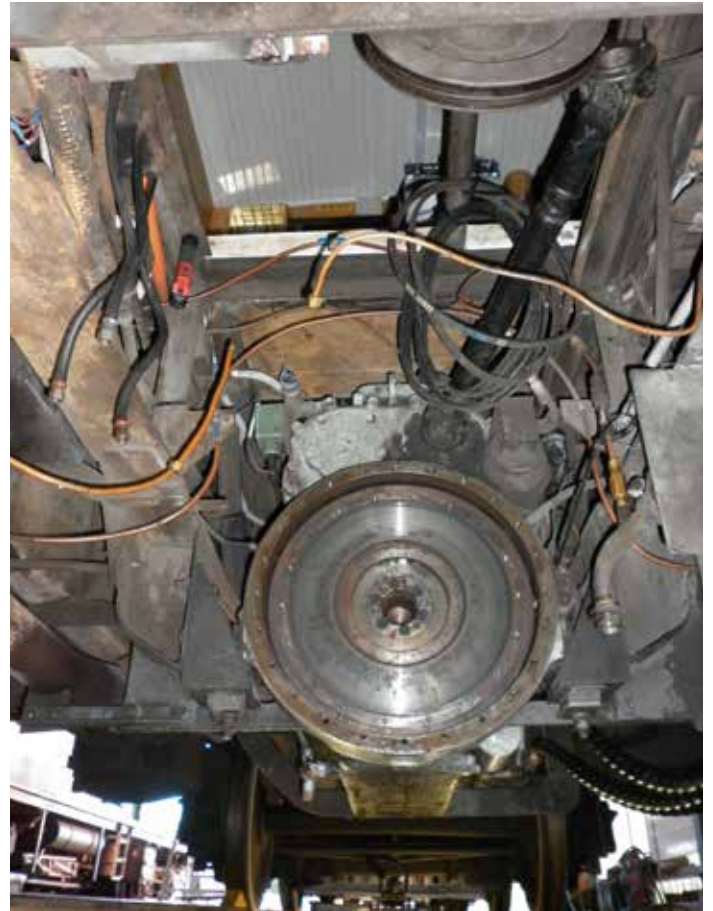
The view beneath the floor of CPH 3 with its transmission removed (looking toward the engine)
