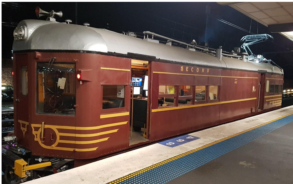
HPC 402 fitted out for overhead wiring inspections
