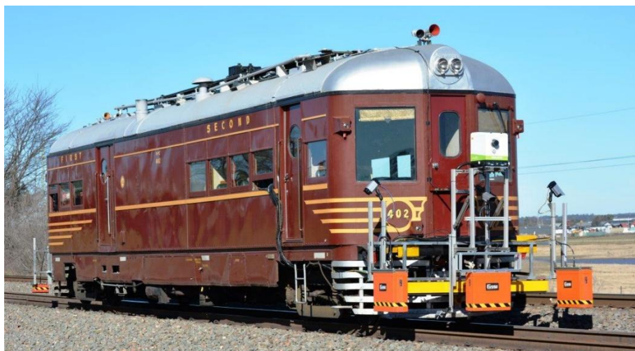
HPC 402 fitted out for ballast testing
