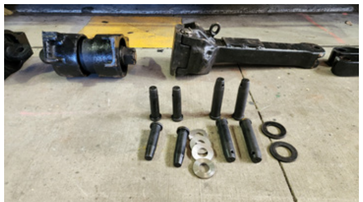
Refurbished spring pack, half-size coupler, coupling pins and plunger bar spring spacers. New plunger bars are just out of sight.
