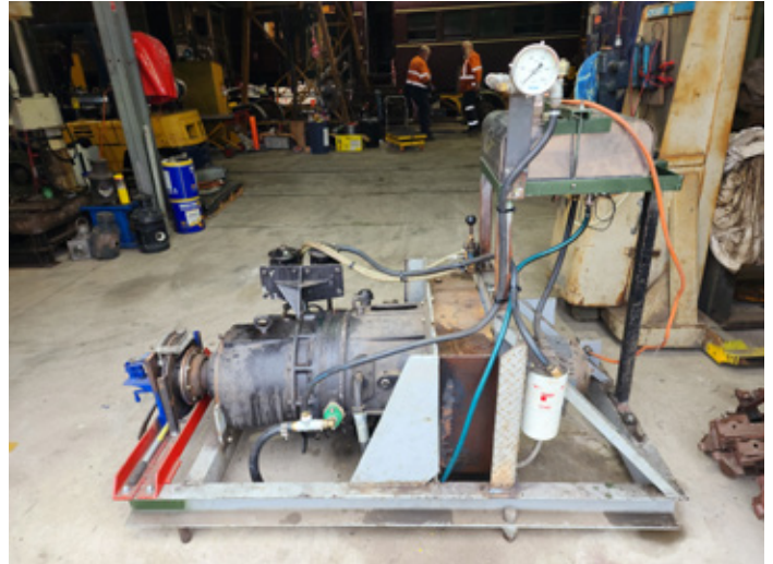
Transmission test rig with the Twin Disc torque converter removed from CPH 3 installed for testing
