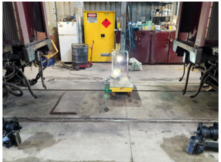
621 and 721 are shown separated, and work to change out worn draw gear is underway, June 2025
