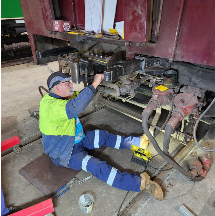
Fitter Gary Delaney works to install a half-size coupler to 721. The new plunger bars can be seen protruding.
