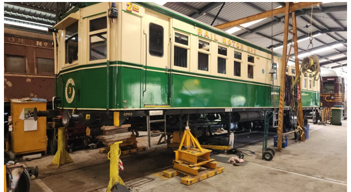
CPH 3 seen raised on hydraulic jacks and its No.2 bogie removed, 17 Sep 2025
