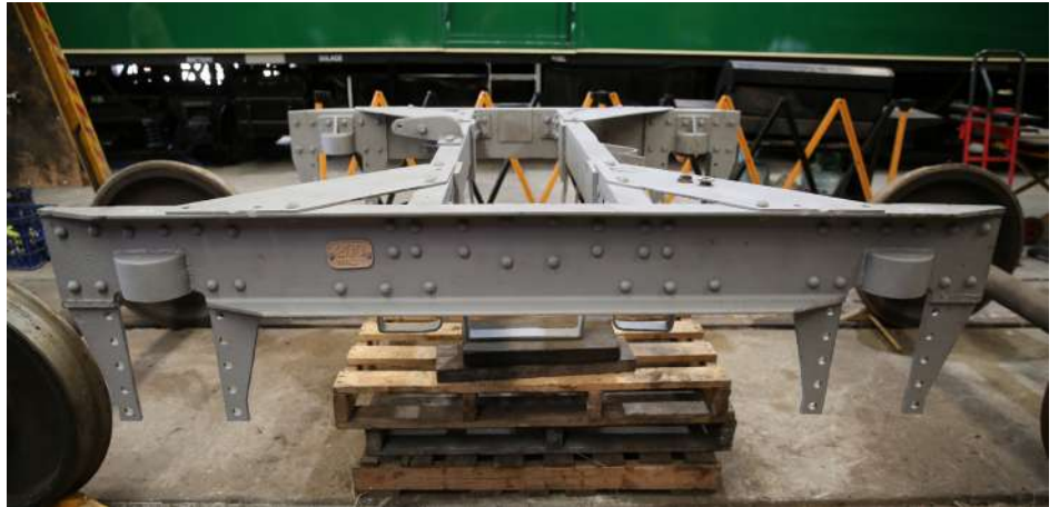
The 2QO bogie frame shown here, after sandblasting back to bare metal, is ready for non-destructive testing to check for structural damage.
