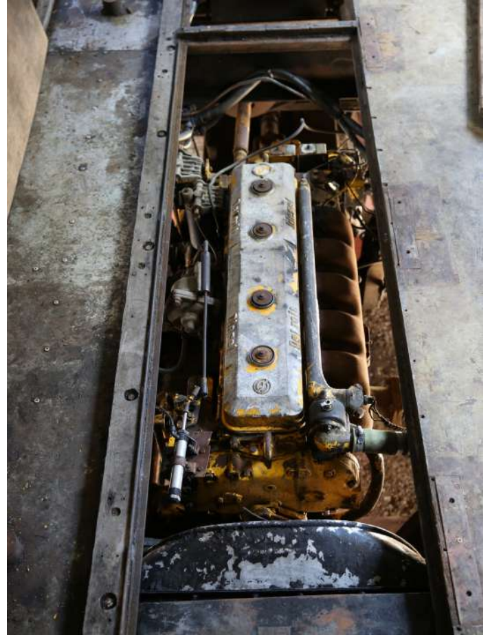
Above: Detroit 6/71 diesel engine in railcar WFP 602, recently cleaned, as seen from above with the floor inspection hatch cover removed (TRMS).
