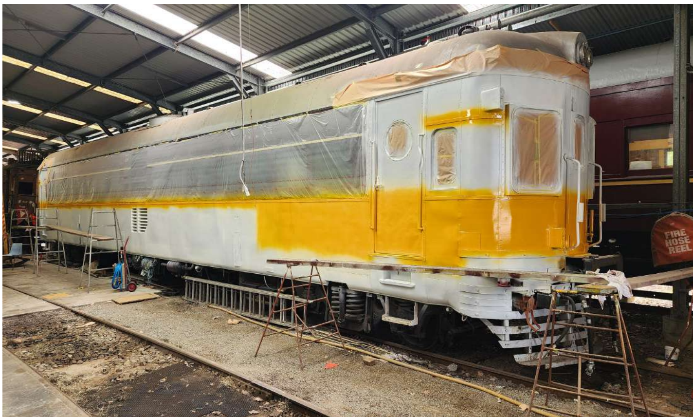
Progress is well underway to restore the heritage livery on NPF 629, with its 'whiskers' to be detailed soon. Note the massive effort Peter Macfarlane has invested in single-handedly masking the windows and in making other preparations (TRMS).
