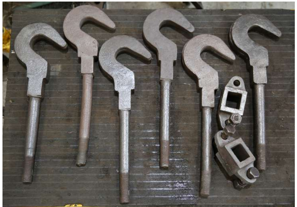
CPH drawbar hooks cleaned and prepared for non-destructive testing.
