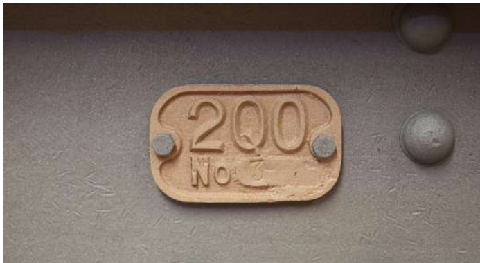
A close-up of the 200 bogie identification plate, stamped No.3. Very few of these bogies, being specific to a CTC trailer car, were made (TRMS).
